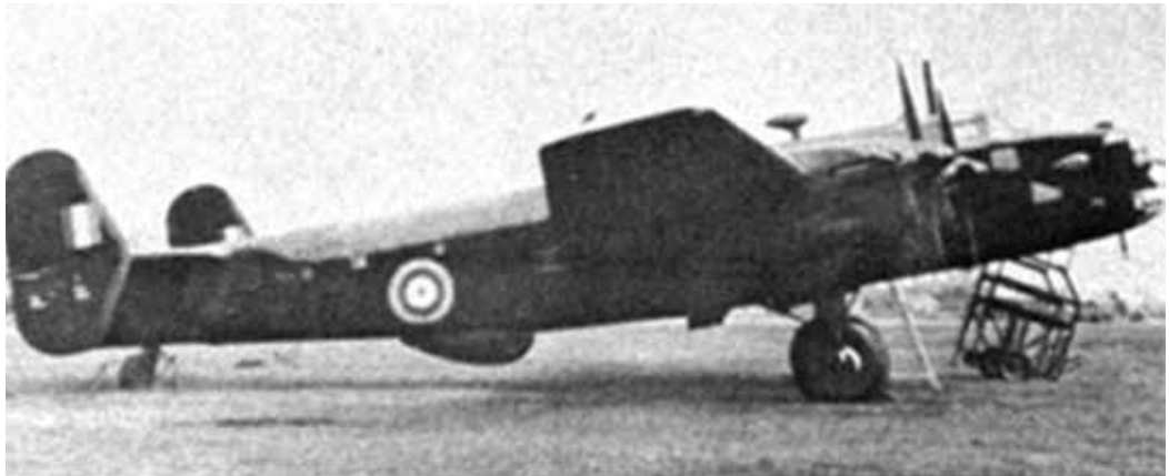
FIGURE 34. H2S S-BAND NAVIGATION AND TARGETING RADAR MOUNTED ON A HANDLEY PAGE HALIFAX BOMBER
