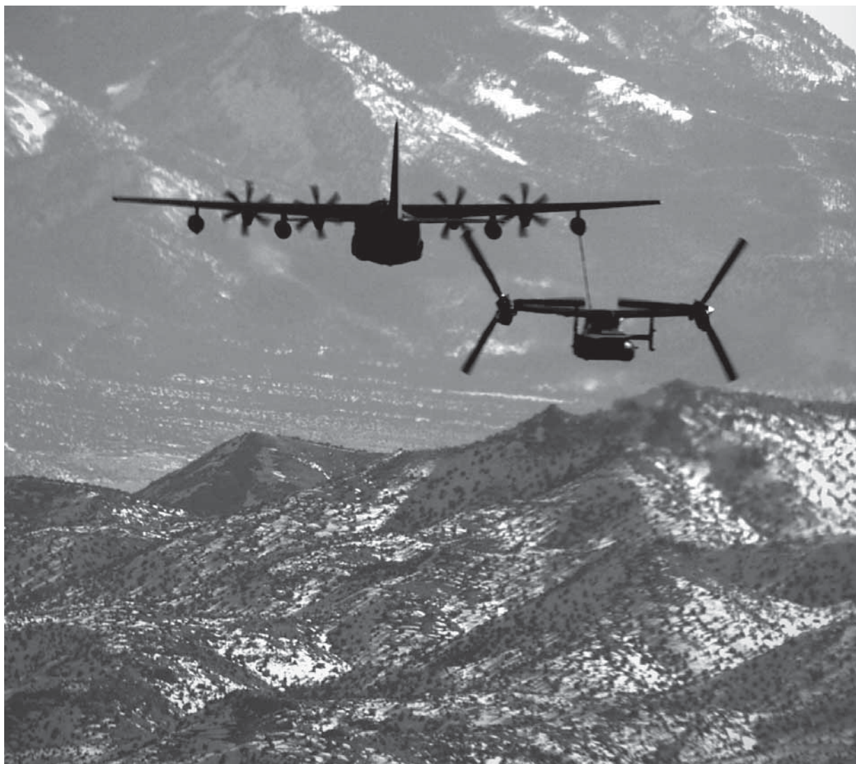
An Air Force MC-130J Commando II refuels an Air Force CV-22 Osprey during a training exercise.
