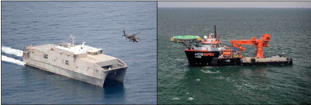
Modified EPF (left) or Multi-Purpose Support Vessels (right) could serve as light tenders. Images courtesy of U.S. Navy and Hornbeck Offshore.
