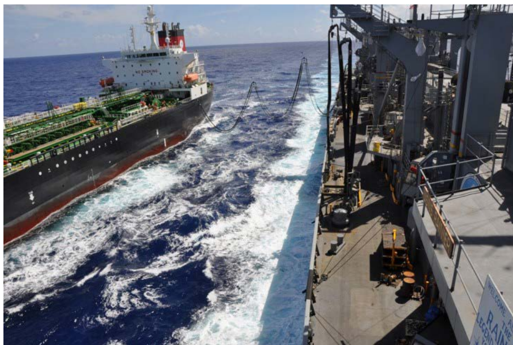
CONSOL tanker MT Empire State and fast combat support ship USNS Rainier conduct CONSOL transfer of fuel. Photo courtesy of U.S. Navy.
