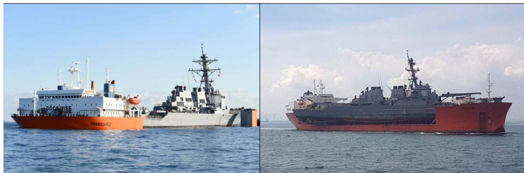
FIGURE 25: ARLEIGH-BURKE-CLASS DDGS LOADED ABOARD FLO/FLO
