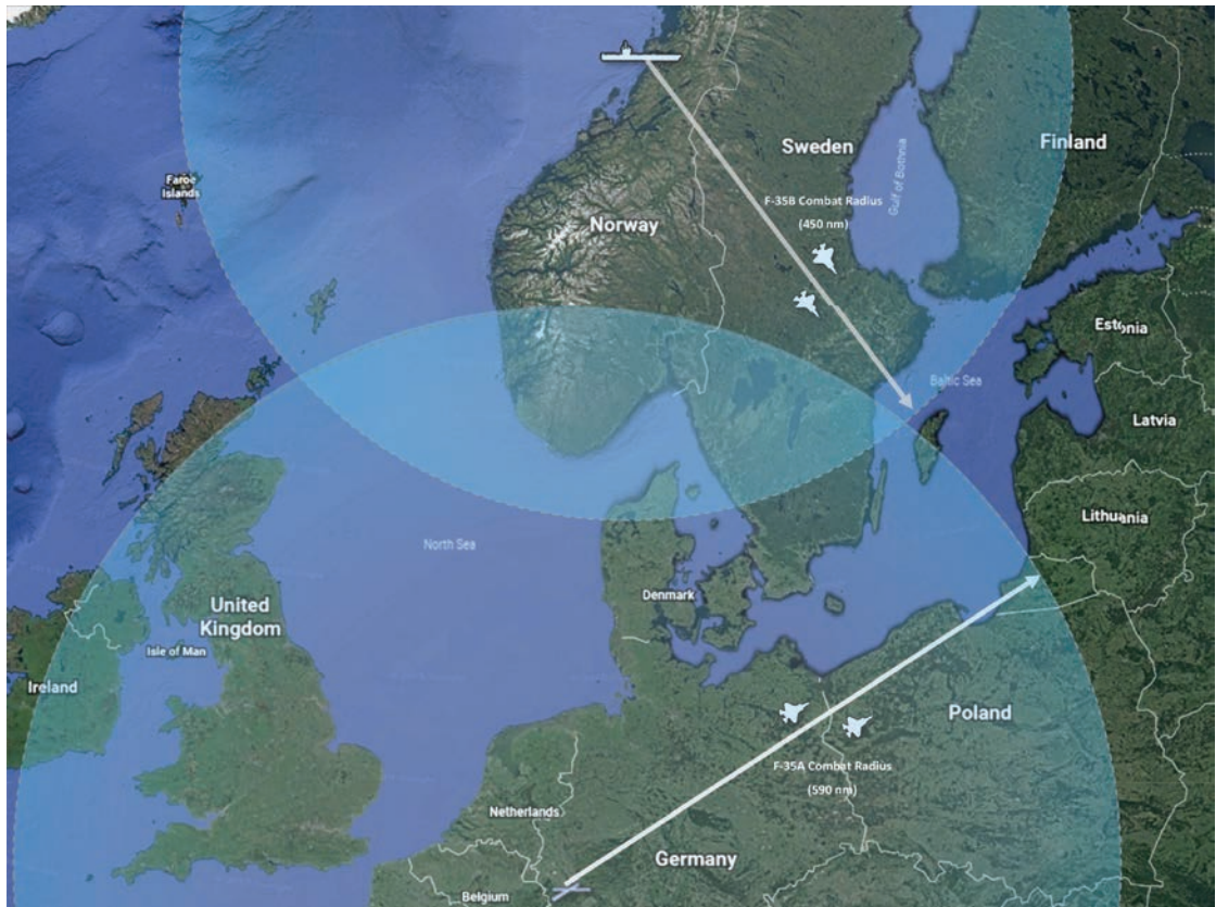
FIGURE 22: ILLUSTRATIVE MAXIMUM PERFECT WORLD COMBAT RADIUS OF THE F-35B AND F-35A ASSUMING NO LOITER TIME OR COMBAT FUEL
