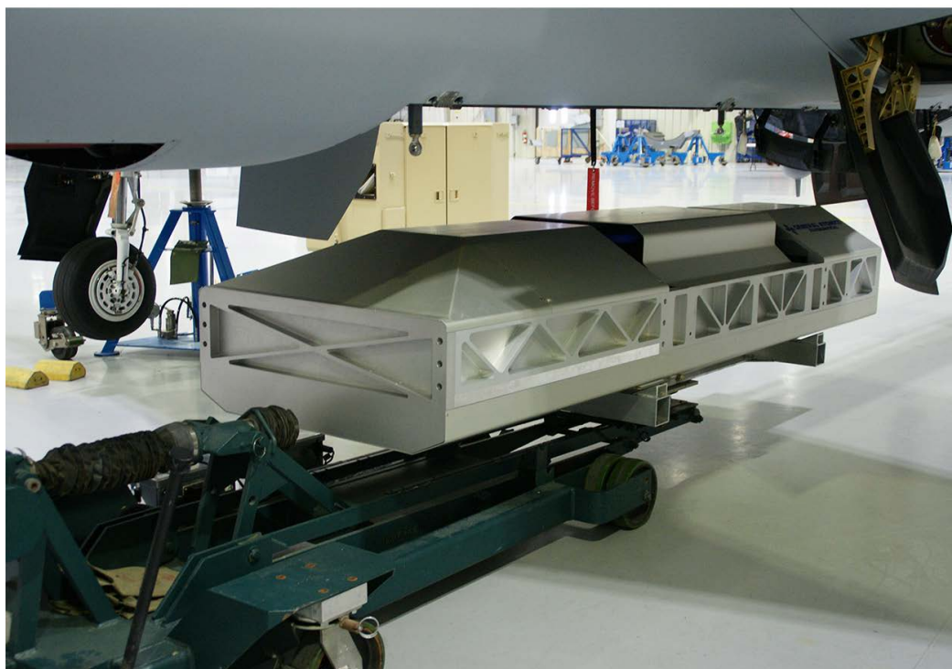
Figures courtesy of General Atomics. These images depict a 100 kW-class Distributed Gain Laser weapon system for integration on a UAV.
