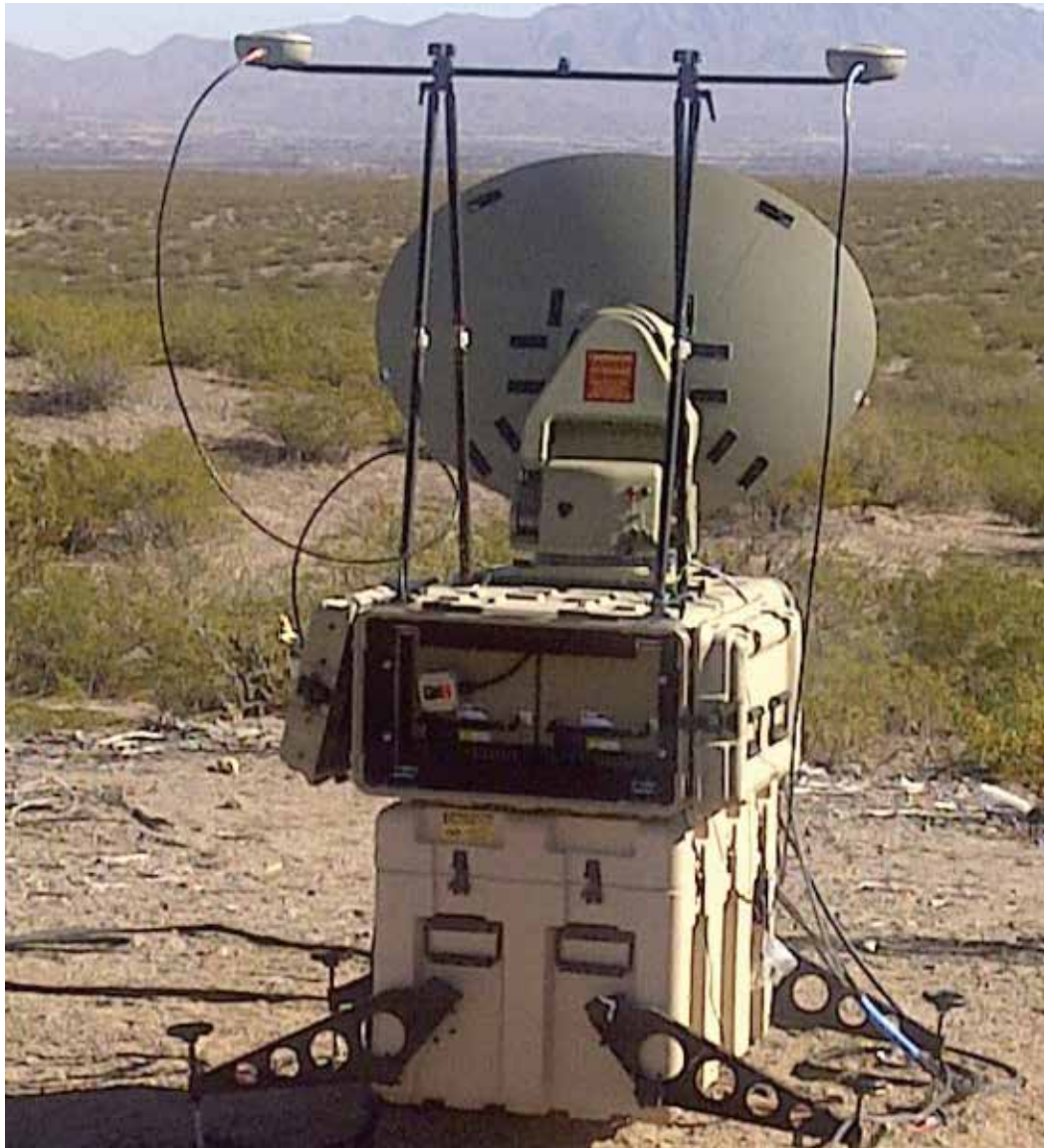
FIGURE 34: TELOS TROPOSCATTER COMMUNICATION SYSTEM
