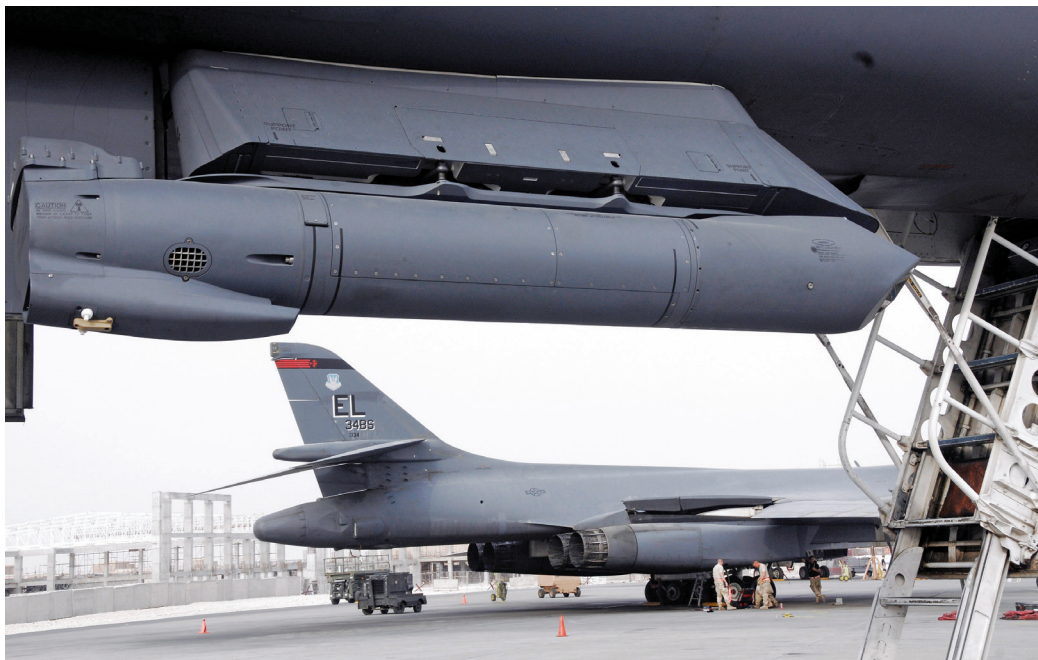
A Sniper Advanced Targeting Pod hangs from the underbelly of a B-1 Lancer. U.S. Air Force photo by Staff Sgt. Darnell Cannady.
