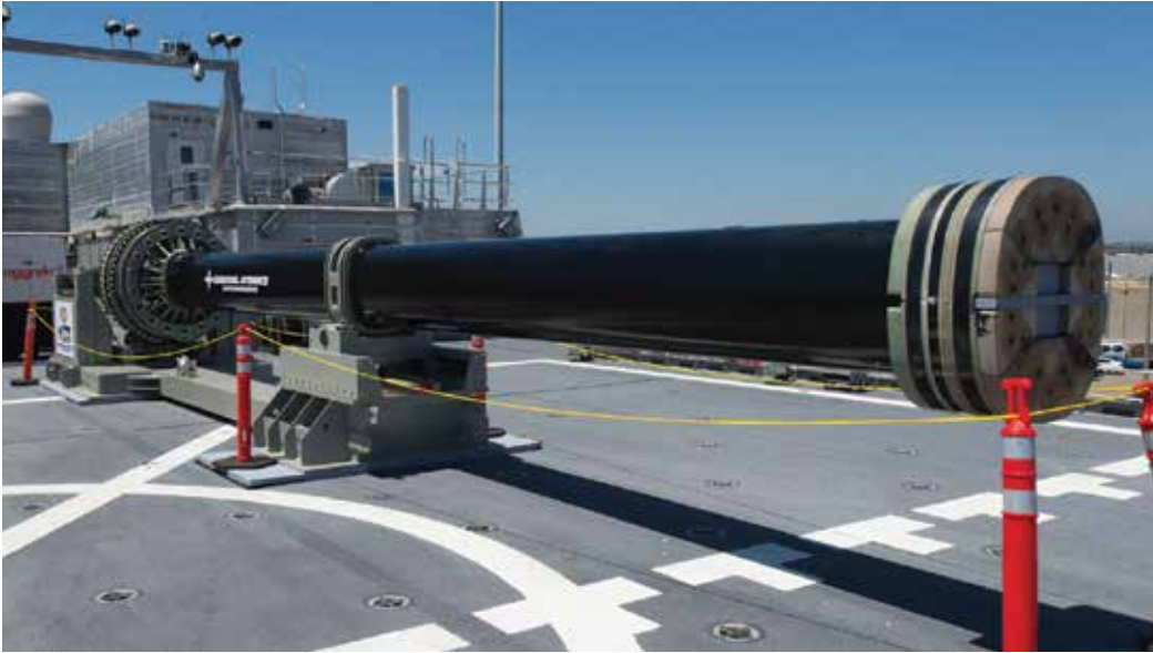
FIGURE 11: THE 32-MJ EMRG BARREL ON USNS MILLINOCKET (T-EPF 3)
