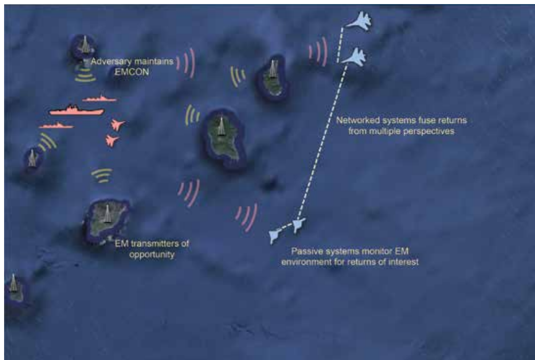
FIGURE 12: PASSIVE RADAR OR PASSIVE COHERENT LOCATION
