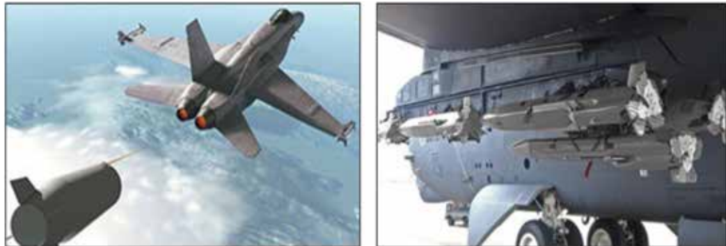
FIGURE 22: TOWED DECOY AND MINIATURE AIR-LAUNCHED DECOY
