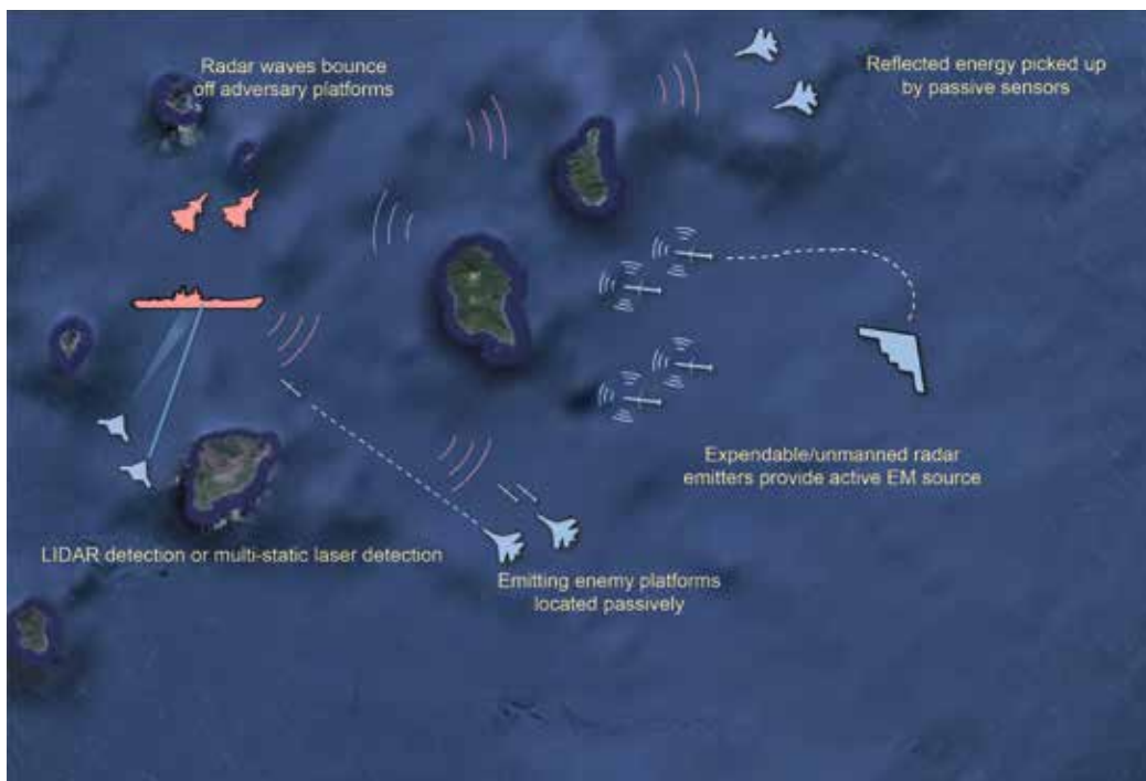
FIGURE 11: CONCEPTS FOR PASSIVE AND MULTISTATIC DETECTION
